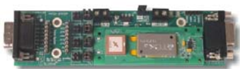
The Bluetooth E-blocks board is at the heart of the training system.
